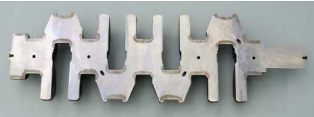
▲ Crankshaft main and pin part, cut surface of heat-treated quenched part
